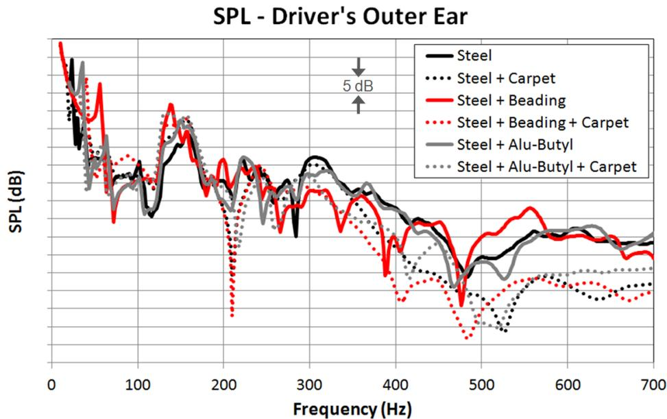
Figure 10: Effect of carpet on various panel construction driver's ear SPL
