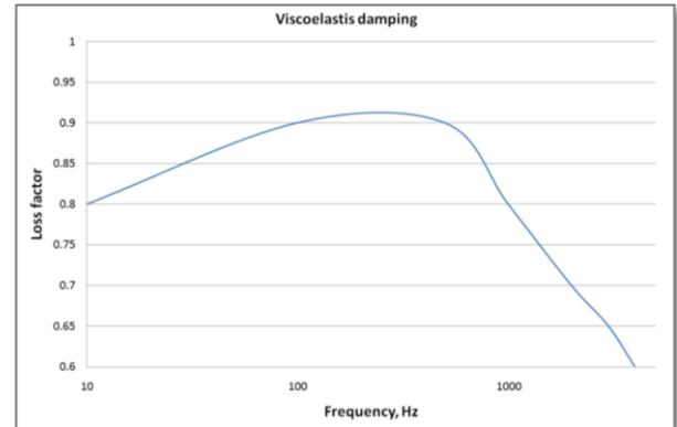
**Figure 3:** Structural damping loss factor of MPM viscoelastic layer
