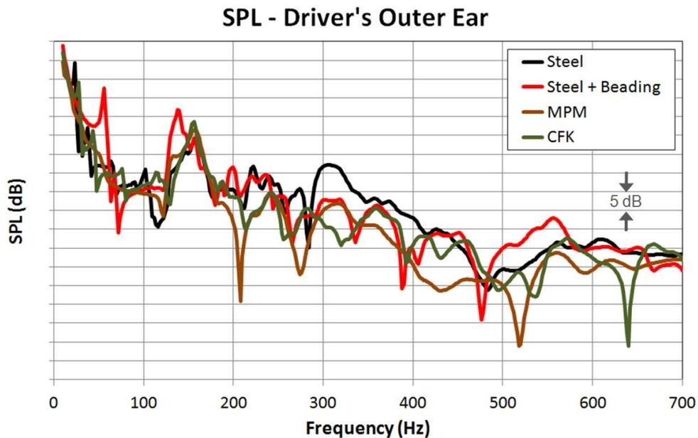
**Figure 5:** Effect of various panel constructions on driver's ear SPL
