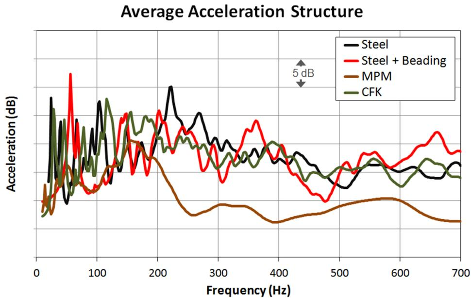
**Figure 4:** Effect of various panel constructions on average acceleration
