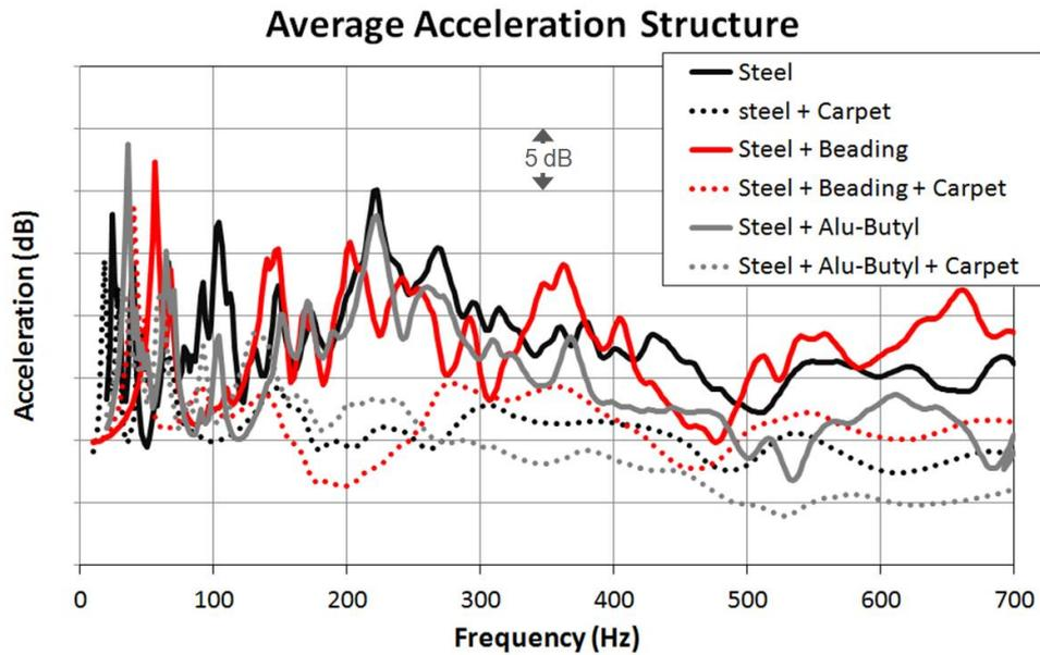
Figure 9: Effect of carpet on various panel construction average acceleration
