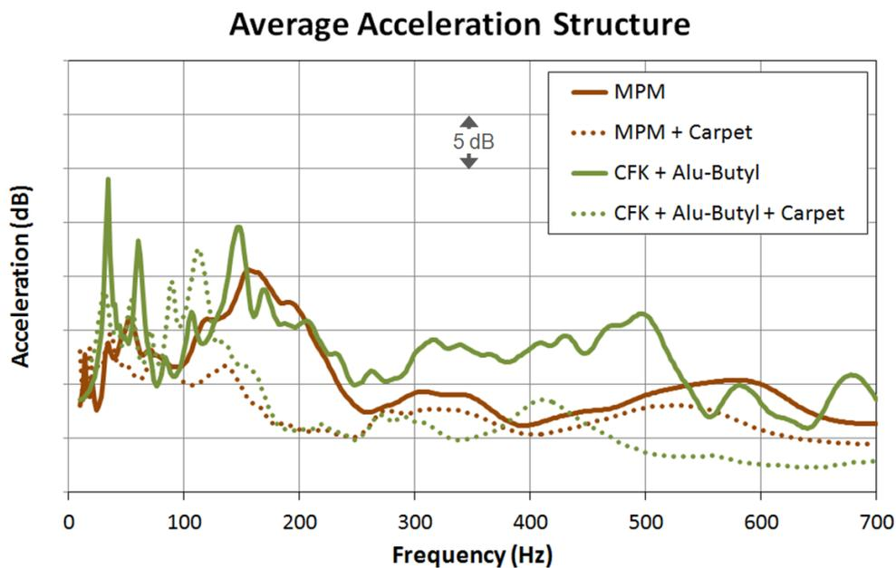
**Figure 11:** Effect on average floor acceleration of carpet on MPM and CFRP
