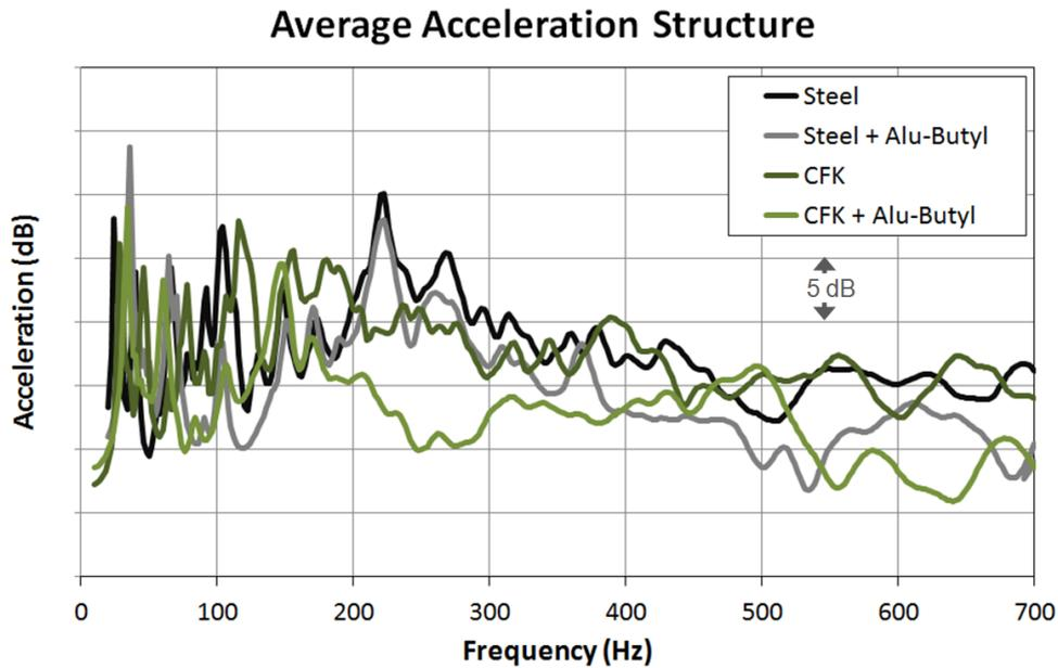
**Figure 7:** Effect of damping patches on car panels average acceleration
