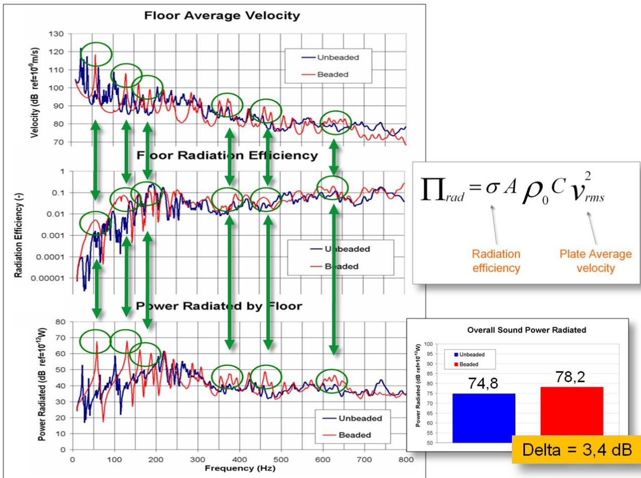
**Figure 6:** Effect of beading on velocity, radiation efficiency and sound power radiated by the floor
