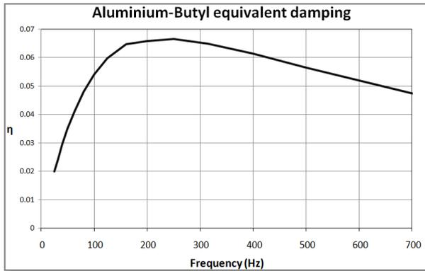
**Figure 2:** Aluminium-Butyl damping patches equivalent damping spectrum
